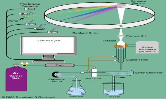
Figure 5. Inductively coupled plasma-atomic emission spectrometry (ICP-AES)
